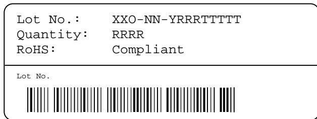
Figure 13: First label on reel: XX = Sensor Type (21 for SHT21), O = Output mode (D = Digital, P = PWM, S = SDM), NN = product revision no., Y = last digit of year, RRR = number of sensors on reel divided by 10 (200 for 2000 units), TTTTT = Traceability Code.
