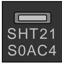
Figure 12 Laser marking on sensor. For details see text.
